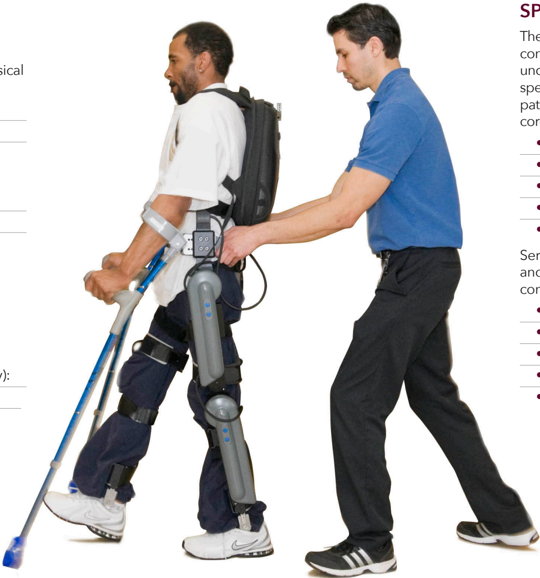
▲ The ReWalk Exoskeleton is a state-of-the-art piece of equipment that combines robotics with human assistance to make walking possible.
